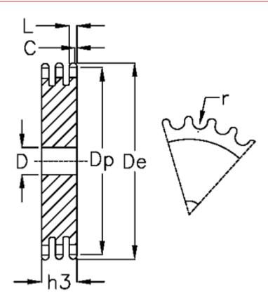
C = 2 D = 30 De = 585.1 Dp = 576.17 For chain size =  $3/4 \times 7/16$ For chain type = 12 B-3 h3 = 49.8 L = 10.8 Number of teeth = 95r = 12.07
